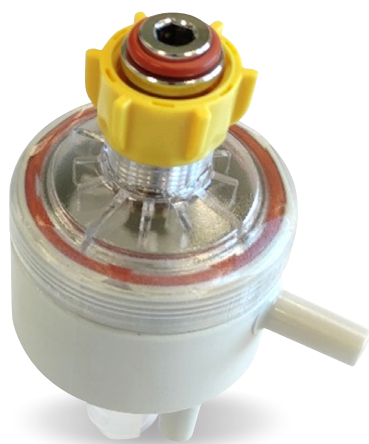
Cover without antibacterial filter Made of polycarbonate and brass (sterilisable at 121°C / 15 min.)
